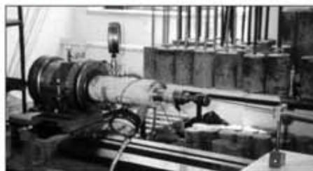
Figure 1. Test set-up showing the arrangement of the bi-axial cell, hydraulic ram, pressure transducer and LVDT.
