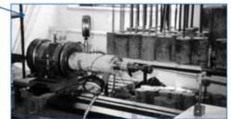
Figure 1. Test set-up showing the arrangement of the bi-axial cell, hydraulic ram, pressure transducer and LVDT.
