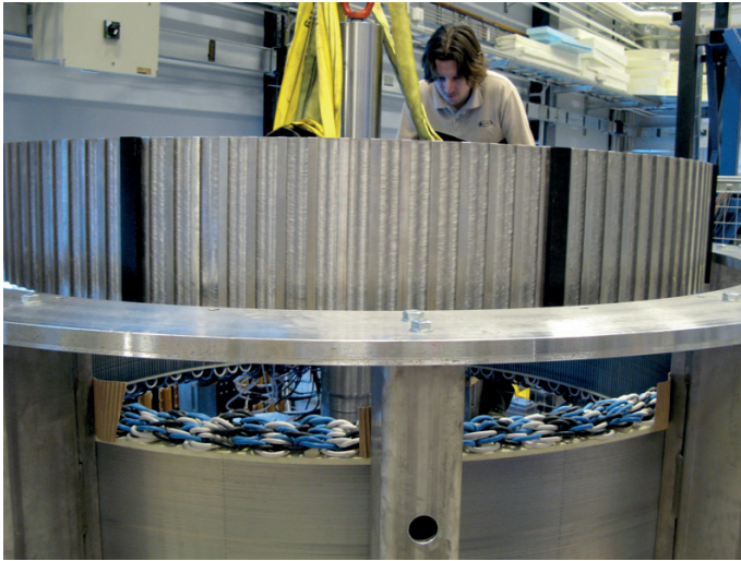
Figure 7.2: The rotor is being lowered into the stator. The milled grooves for the magnets are clearly seen on the rotor ring.
