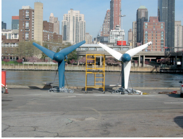
Figure 2.1: Two of the turbines deployed in New York City’s East River. The diameter of the turbine is 5 m (used with permission).
