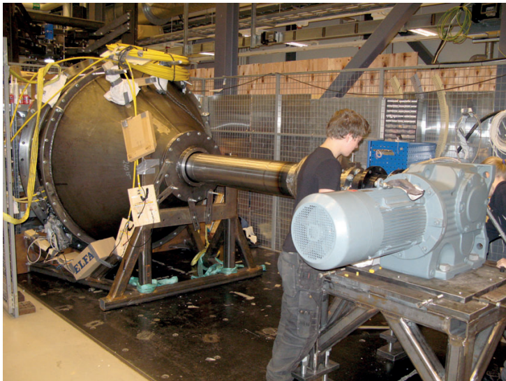
Figure 8.8: The machine in horizontal position for laboratory experiments, connected to a motor drive system and a torque measuring system (from Paper VIII).
