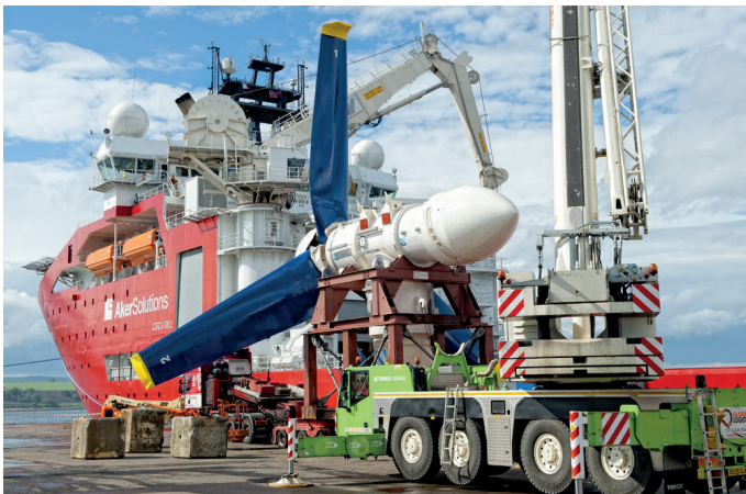
Figure 5.1: A picture of the 1 MW AR1000 series turbine by Atlantis Resource Corporation before deployment (used with permission).
