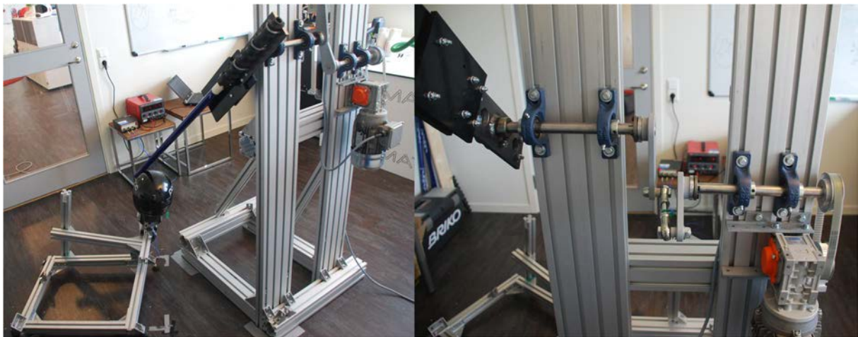
Figure 1. To the left, the test device and the used test setup where the rotating pole impacted the helmet on the left side of the centerline. To the right, a close-up on the drive chain with the motor in bottom right corner and with the attached gearbox which drives the two drive shafts that are connected with asymmetrical mounted rods. (Reproduced from [99].)
