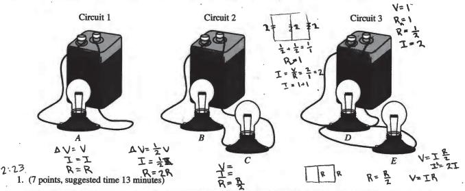
In the three circuits shown above, the batteries are all identical, and the lightbulbs are all identical. In circuit 1 a single lightbulb is connected to the battery. In circuits 2 and 3, two lightbulbs are connected to the battery in different ways, as shown. The lightbulbs are labeled A-E.
