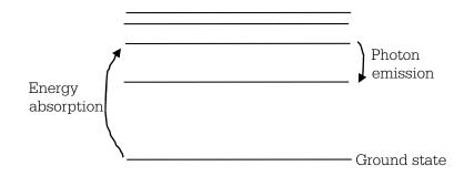
Atoms in the ground state absorb energy from the electricity delivered to the lamp. The atoms enter an excited state. Then the atoms emit photons as they drop to a lower energy state.
