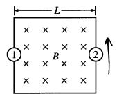
For indicating that current flows upward in bulb 2 or counterclockwise around the loop 1 point
