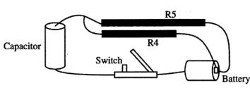
The student uses resistors R4 and R5 to build a circuit using wire, a 1.5 V battery, an uncharged 10  $\mu$ F capacitor, and an open switch, as shown above.
