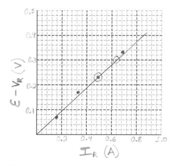
(e) Use your straight line to calculate the value of the resistance of the wire sample.  $slope = \frac{0.3 - 0.23}{0.64 - 0.49} = \frac{0.07}{0.15} = 0.4667 \Omega = \frac{E - VR}{IR} = \Gamma$
