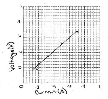
(e) Use your straight line to calculate the value of the resistance of the wire sample.
