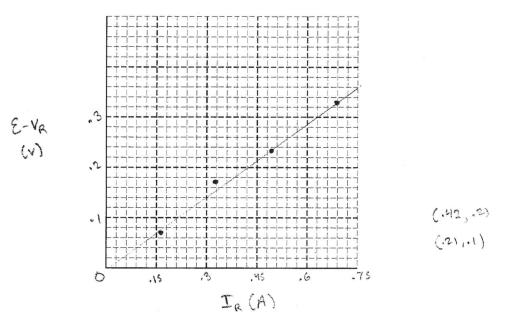
(e) Use your straight line to calculate the value of the resistance of the wire sample.
