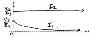
The circuit is constructed using an ideal 1.5 V battery, an 80  $\mu$ F capacitor, and resistors  $R_1 = 150 \Omega$  and  $R_2 = 100 \Omega$ . The switch is closed, allowing the capacitor to fully charge. The switch is then opened, allowing the capacitor to discharge.
