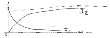
The circuit is constructed using an ideal 1.5 V battery, an 80  $\mu$ F capacitor, and resistors  $R_1 = 150 \Omega$  and  $R_2 = 100 \Omega$ . The switch is closed, allowing the capacitor to fully charge. The switch is then opened, allowing the capacitor to discharge.
