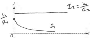
The circuit is constructed using an ideal 1.5 V battery, an 80  $\mu$ F capacitor, and resistors  $R_1$  = 150  $\Omega$  and  $R_2$  = 100  $\Omega$ . The switch is closed, allowing the capacitor to fully charge. The switch is then opened, allowing the capacitor to discharge.
