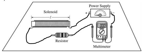
For connections that create a circuit with the power supply, solenoid, and resistor in series with each other
