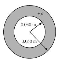
A nonconducting hollow sphere of inner radius 0.030 m and outer radius 0.050 m carries a positive volume charge density  $\rho$ , as shown in the figure above. The charge density  $\rho$  of the sphere is given as a function of the distance r from the center of the sphere, in meters, by the following.
