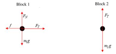
**Scoring note**: Examples of appropriate labels for the force due to gravity include:  $F_G$ ,  $F_{\rm g}$  ,  $F_{\rm grav}$  , W , mg , Mg , "grav force," "F Earth on block," "F on block by Earth,"  $F_{\rm Earth\ on\ block}$  ,  $F_{\rm E,Block}$  ,  $F_{\rm Block,E}$  . The labels G or g are not appropriate labels for the force due to gravity.  $F_n$ ,  $F_N$ , N, "normal force," "ground force," or similar labels may be used for the normal force.
