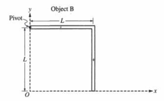
Object B of total mass  $\underline{M}$  is formed by attaching two thin, uniform, identical rods of length L at a right angle to each other. Object B is held in place, as shown above. Express your answers in part (b) in terms of L.
