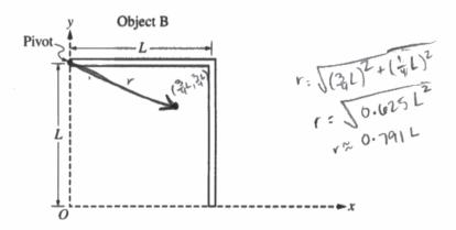
Object B of total mass M is formed by attaching two thin, uniform, identical rods of length L at a right angle to each other. Object B is held in place, as shown above. Express your answers in part (b) in terms of L.
