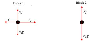
**Scoring note**: Examples of appropriate labels for the force due to gravity include:  $F_{\rm G}$ ,  $F_{\rm g}$ ,  $F_{\rm grav}$ , W, mg, Mg, "grav force," "F Earth on block," "F on block by Earth,"  $F_{\rm Earth\ on\ block}$ ,  $F_{\rm E,Block}$ ,  $F_{\rm Block,E}$ . The labels G or g are not appropriate labels for the force due to gravity.  $F_n$ ,  $F_N$ , N, "normal force," "ground force," or similar labels may be used for the normal force.
