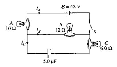
(d) Now consider a similar circuit with an uncharged 5.0 μF capacitor instead of the inductor, as shown above. The switch is again closed at time t = 0. On the axes below, sketch the magnitude of the potential difference V<sub>cap</sub> across the capacitor as a function of time, from immediately after the switch is closed until a long time after the switch is closed.
