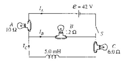
Now a switch S and a 5.0 mH inductor are added to the circuit, as shown above. The switch is closed at time t = 0.
