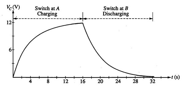
(d) Draw a schematic diagram of the RC circuit that you constructed that would produce the graph above. Clearly indicate switch positions A and B on your circuit diagram and include whatever other devices you need to measure the voltage across the capacitor to obtain the above plot. Label each component in your diagram.
