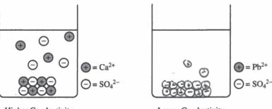
Higher Conductivity Solution Lower Conductivity Solution
