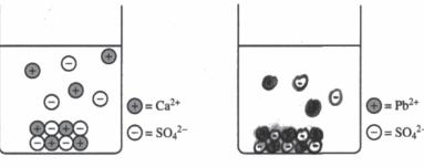
Higher Conductivity Solution Lower Conductivity Solution
