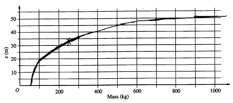
ii. Using your best-fit curve, determine the distance x traveled by the projectile if 250 kg is placed in the counterweight bucket.
