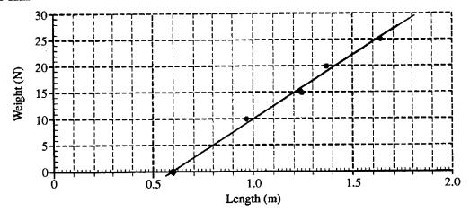
(b) Use the best-fit line you sketched in part (a) to determine an experimental value for the spring constant k of the cord.
