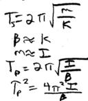
To determine the torsion constant  $\beta$  of the rod, disks of different, known values of rotational inertia are attached to the rod, and the data below are obtained from the resulting oscillations.
