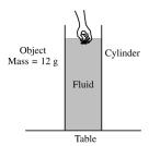
In an experiment, students used video analysis to track the motion of an object falling vertically through a fluid in a glass cylinder. The object of m = 12 g is released from rest at the top of the column of fluid, as shown above. The data for the speed v of the falling object as a function of time t are graphed on the grid below. The dashed curve represents the best fit chosen by the students for these data.
