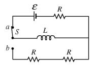
In the circuit above, all of the resistors have the same resistance R. Switch S has been in position a for a very long time.
